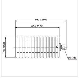
RF Solution offer a wide selection of Coaxial Fixed Termination (Dummy Load) for global customers. CT-50W-RA3885-SJ-18G is Coaxial а Termination (Dummy Load) in Frequency Range of DC~18.0 GHz. It is made of high quality materials under a high standard, the Connector Type of this product is SMA-M (J), VSWR Max is 1.40 and Impedance is 50  $\Omega$ . The component has a good working performance and stability, it is ideal for handling a Power of 50 W.
