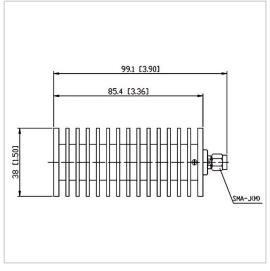
RF Solution offer a wide selection of Coaxial Fixed Termination (Dummy Load) for global customers. CT-50W-RA3885-SJ-12.4G is a Coaxial Fixed Termination (Dummy Load) in Frequency Range of DC~12.4 GHz. It is made of high quality materials under a high standard, the Connector Type of this product is SMA-M (J), VSWR Max is 1.35 and Impedance is 50  $\Omega$ . The component has a good working performance and stability, it is ideal for handling a Power of 50 W.
