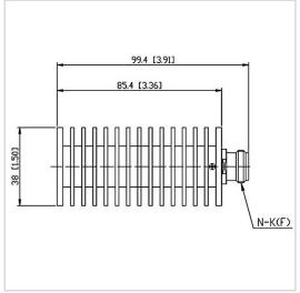
RF Solution offer a wide selection of Coaxial Fixed Termination (Dummy Load) for global customers. CT-50W-RA3885-NK-12.4G is Coaxial Termination (Dummy Load) in Frequency Range of DC~12.4 GHz. It is made of high quality materials under a high standard, the Connector Type of this product is N-F (K), VSWR Max is 1.30 and Impedance N-K(F) is 50  $\Omega$ . The component has a good working performance and stability, it is ideal for handling a Power of 50 W.
