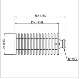
RF Solution offer a wide selection of Coaxial Fixed Termination (Dummy Load) for global customers. CT-50W-RA3885-NK-10G is Coaxial Fixed Termination (Dummy Load) in Frequency Range of DC~10.0 GHz. It is made of high quality materials under a high standard, the Connector Type of this product is N-F (K), VSWR Max is 1.30 and Impedance  $\frac{N-K(F)}{\Gamma}$  is 50  $\Omega$ . The component has a good working performance and stability, it is ideal for handling a Power of 50 W.
