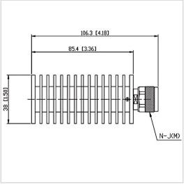
RF Solution offer a wide selection of Coaxial Fixed Termination (Dummy Load) for global customers. CT-50W-RA3885-NJ-18G is Coaxial Fixed Termination (Dummy Load) in Frequency Range of DC~18.0 GHz. It is made of high quality materials under a high standard, the Connector Type of this product is N-M (J), VSWR Max is 1.40 and Impedance is 50  $\Omega$ . The component has a good working performance and stability, it is ideal for handling a Power of 50 W.
