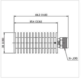
RF Solution offer a wide selection of Coaxial Fixed Termination (Dummy Load) for global customers. CT-50W-RA3885-NJ-12.4G is a Coaxial Fixed Termination (Dummy Load) in Frequency Range of DC~12.4 GHz. It is made of high quality materials under a high standard, the Connector Type of this product is N-M (J), VSWR Max is 1.35 and Impedance is 50  $\Omega$ . The component has a good working performance and stability, it is ideal for handling a Power of 50 W.
