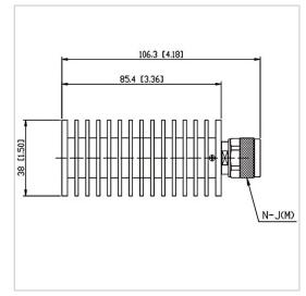
RF Solution offer a wide selection of Coaxial Fixed Termination (Dummy Load) for global customers. CT-50W-RA3885-NJ-10G is a Coaxial Fixed Termination (Dummy Load) in Frequency Range of DC~10.0 GHz. It is made of high quality materials under a high standard, the Connector Type of this product is N-M (J), VSWR Max is 1.30 and Impedance is 50  $\Omega$ . The component has a good working performance and stability, it is ideal for handling a Power of 50 W.
