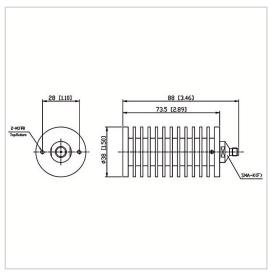
RF Solution offer a wide selection of Coaxial Fixed Termination (Dummy Load) for global customers. CT-50W-RA3873-SK-4G is Coaxial Fixed а Termination (Dummy Load) in Frequency Range of DC~4.0 GHz. It is made of high quality materials under a high standard, the Connector Type of this product is SMA-F (K), VSWR Max is 1.20 and Impedance is 50  $\Omega$ . The component has a good working performance and stability, it is ideal for handling a Power of 50 W.
