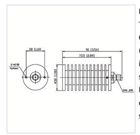
RF Solution offer a wide selection of Coaxial Fixed Termination (Dummy Load) for global customers. CT-50W-RA3873-SJ-8G is a Coaxial Fixed Termination (Dummy Load) in Frequency Range of DC~8.0 GHz. It is made of high quality materials under a high standard, the Connector Type of this product is SMA-M (J), VSWR Max is 1.30 and Impedance is 50  $\Omega$ . The component has a good working performance and stability, it is ideal for handling a Power of 50 W.
