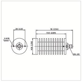
RF Solution offer a wide selection of Coaxial Fixed Termination (Dummy Load) for global customers. CT-50W-RA3873-SJ-6G is a Coaxial Fixed Termination (Dummy Load) in Frequency Range of DC $\sim$ 6.0 GHz. It is made of high quality materials under a high standard, the Connector Type of this product is SMA-M (J), VSWR Max is 1.25 and Impedance is 50  $\Omega$ . The component has a good working performance and stability, it is ideal for handling a Power of 50 W.
