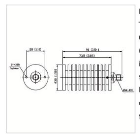
RF Solution offer a wide selection of Coaxial Fixed Termination (Dummy Load) for global customers. CT-50W-RA3873-SJ-4G is a Coaxial Fixed Termination (Dummy Load) in Frequency Range of DC~4.0 GHz. It is made of high quality materials under a high standard, the Connector Type of this product is SMA-M (J), VSWR Max is 1.20 and Impedance is 50  $\Omega$ . The component has a good working performance and stability, it is ideal for handling a Power of 50 W.
