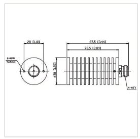
RF Solution offer a wide selection of Coaxial Fixed Termination (Dummy Load) for global customers. CT-50W-RA3873-NK-4G is Coaxial Fixed а Termination (Dummy Load) in Frequency Range of DC~4.0 GHz. It is made of high quality materials under a high standard, the Connector Type of this product is N-F (K), VSWR Max is 1.20 and Impedance is 50  $\Omega$ . The component has a good working performance and stability, it is ideal for handling a Power of 50 W.
