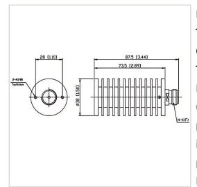
RF Solution offer a wide selection of Coaxial Fixed Termination (Dummy Load) for global customers. CT-50W-RA3873-NK-3G is a Coaxial Fixed Termination (Dummy Load) in Frequency Range of DC~3.0 GHz. It is made of high quality materials under a high standard, the Connector Type of this product is N-M (J), VSWR Max is 1.20 and Impedance is 50  $\Omega$ . The component has a good working performance and stability, it is ideal for handling a Power of 50 W.
