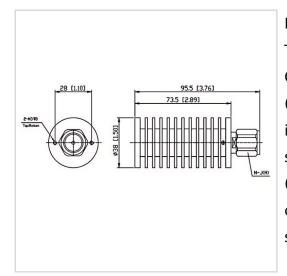
RF Solution offer a wide selection of Coaxial Fixed Termination (Dummy Load) for global customers. CT-50W-RA3873-NJ-6G is a Coaxial Fixed Termination (Dummy Load) in Frequency Range of DC~6.0 GHz. It is made of high quality materials under a high standard, the Connector Type of this product is N-M (J), VSWR Max is 1.25 and Impedance is 50  $\Omega$ . The component has a good working performance and stability, it is ideal for handling a Power of 50 W.
