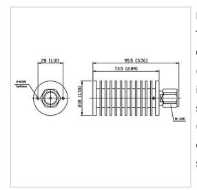
RF Solution offer a wide selection of Coaxial Fixed Termination (Dummy Load) for global customers. CT-50W-RA3873-NJ-4G is a Coaxial Fixed Termination (Dummy Load) in Frequency Range of DC~4.0 GHz. It is made of high quality materials under a high standard, the Connector Type of this product is N-M (J), VSWR Max is 1.20 and Impedance is 50  $\Omega$ . The component has a good working performance and stability, it is ideal for handling a Power of 50 W.
