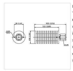
RF Solution offer a wide selection of Coaxial Fixed Termination (Dummy Load) for global customers. CT-50W-RA3873-NJ-3G is a Coaxial Fixed Termination (Dummy Load) in Frequency Range of DC $\sim$ 3.0 GHz. It is made of high quality materials under a high standard, the Connector Type of this product is N-M (J), VSWR Max is 1.20 and Impedance is 50  $\Omega$ . The component has a good working performance and stability, it is ideal for handling a Power of 50 W.
