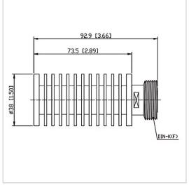
RF Solution offer a wide selection of Coaxial Fixed Termination (Dummy Load) for global customers. CT-50W-RA3873-DINK-6G is a Coaxial Fixed Termination (Dummy Load) in Frequency Range of DC $\sim$ 6.0 GHz. It is made of high quality materials under a high standard, the Connector Type of this product is DIN-F (K), VSWR Max is 1.30 and Impedance is 50  $\Omega$ . The component has a good working performance and stability, it is ideal for handling a Power of 50 W.
