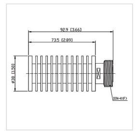
RF Solution offer a wide selection of Coaxial Fixed Termination (Dummy Load) for global customers. CT-50W-RA3873-DINK-4G is a Coaxial Fixed Termination (Dummy Load) in Frequency Range of DC~4.0 GHz. It is made of high quality materials under a high standard, the Connector Type of this product is DIN-F (K), VSWR Max is 1.25 and Impedance is 50  $\Omega$ . The component has a good working performance and stability, it is ideal for handling a Power of 50 W.
