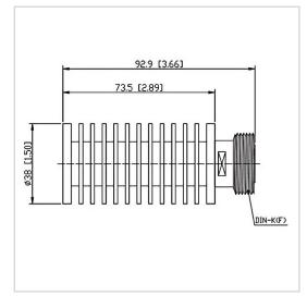
RF Solution offer a wide selection of Coaxial Fixed Termination (Dummy Load) for global customers. CT-50W-RA3873-DINK-3G is a Coaxial Fixed Termination (Dummy Load) in Frequency Range of DC~3.0 GHz. It is made of high quality materials under a high standard, the Connector Type of this product is DIN-F (K), VSWR Max is 1.20 and Impedance is 50  $\Omega$ . The component has a good working performance and stability, it is ideal for handling a Power of 50 W.
