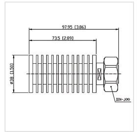
RF Solution offer a wide selection of Coaxial Fixed Termination (Dummy Load) for global customers. CT-50W-RA3873-DINJ-4G is a Coaxial Fixed Termination (Dummy Load) in Frequency Range of DC~4.0 GHz. It is made of high quality materials under a high standard, the Connector Type of this product is DIN-M (J), VSWR Max is 1.25 and Impedance is 50  $\Omega$ . The component has a good working performance and stability, it is ideal for handling a Power of 50 W.
