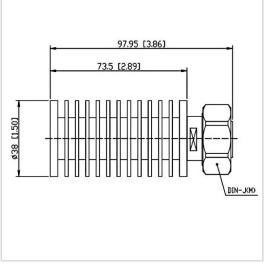
RF Solution offer a wide selection of Coaxial Fixed Termination (Dummy Load) for global customers. CT-50W-RA3873-DINJ-3G is a Coaxial Fixed Termination (Dummy Load) in Frequency Range of DC $\sim$ 3.0 GHz. It is made of high quality materials under a high standard, the Connector Type of this product is DIN-M (J), VSWR Max is 1.20 and Impedance is 50  $\Omega$ . The component has a good working performance and stability, it is ideal for handling a Power of 50 W.
