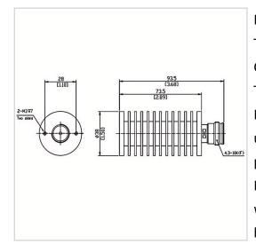
RF Solution offer a wide selection of Coaxial Fixed Termination (Dummy Load) for global customers. CT-50W-RA3873-4310K-6G is a Coaxial Fixed Termination (Dummy Load) in Frequency Range of DC~6.0 GHz. It is made of high quality materials under a high standard, the Connector Type of this product is 4.3-10-F (K), VSWR Max is 1.30 and Impedance is 50  $\Omega$ . The component has a good working performance and stability, it is ideal for handling a Power of 50 W.
