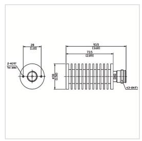
RF Solution offer a wide selection of Coaxial Fixed Termination (Dummy Load) for global customers. CT-50W-RA3873-4310K-4G is a Coaxial Fixed Termination (Dummy Load) in Frequency Range of DC~4.0 GHz. It is made of high quality materials under a high standard, the Connector Type of this product is 4.3-10-F (K), VSWR Max is 1.20 and Impedance is 50  $\Omega$ . The component has a good working performance and stability, it is ideal for handling a Power of 50 W.
