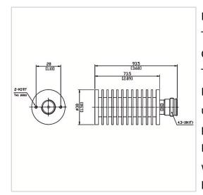
RF Solution offer a wide selection of Coaxial Fixed Termination (Dummy Load) for global customers. CT-50W-RA3873-4310K-3G is a Coaxial Fixed Termination (Dummy Load) in Frequency Range of DC~3.0 GHz. It is made of high quality materials under a high standard, the Connector Type of this product is 4.3-10-F (K), VSWR Max is 1.20 and Impedance is 50  $\Omega$ . The component has a good working performance and stability, it is ideal for handling a Power of 50 W.
