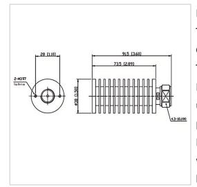
RF Solution offer a wide selection of Coaxial Fixed Termination (Dummy Load) for global customers. CT-50W-RA3873-4310J-6G is a Coaxial Fixed Termination (Dummy Load) in Frequency Range of DC~6.0 GHz. It is made of high quality materials under a high standard, the Connector Type of this product is 4.3-10-M (J), VSWR Max is 1.30 and Impedance is 50  $\Omega$ . The component has a good working performance and stability, it is ideal for handling a Power of 50 W.
