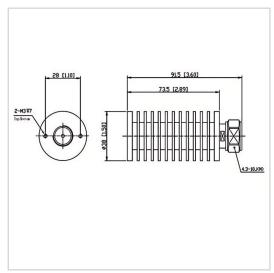
RF Solution offer a wide selection of Coaxial Fixed Termination (Dummy Load) for global customers. CT-50W-RA3873-4310J-3G is a Coaxial Fixed Termination (Dummy Load) in Frequency Range of DC~3.0 GHz. It is made of high quality materials under a high standard, the Connector Type of this product is 4.3-10-M (J), VSWR Max is 1.20 and Impedance is 50  $\Omega$ . The component has a good working performance and stability, it is ideal for handling a Power of 50 W.
