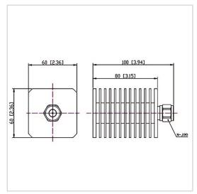
RF Solution offer a wide selection of Coaxial Low PIM Termination for global customers. CT-50W-FH6080-IP65-NJ-3G is a Coaxial Low PIM Termination in Frequency Range of DC $\sim$ 3.0 GHz. It is made of high quality materials under a high standard, the Connector Type of this product is N-M (J), VSWR Max is 1.20 and Impedance is 50  $\Omega$ . The component has a good working performance and stability, it is ideal for handling a Power of 50 W.
