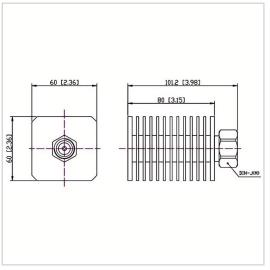
RF Solution offer a wide selection of Coaxial Low PIM Termination for global customers. CT-50W-FH6080-IP65-DINJ-3G is а Coaxial Low Termination in Frequency Range of DC~3.0 GHz. It is made of high quality materials under a high standard, the Connector Type of this product is DIN-M (J), VSWR Max is 1.20 and Impedance is 50  $\Omega$ . The component has a good working performance and stability, it is ideal for handling a Power of 50 W.
