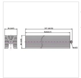
RF Solution offer a wide selection of Coaxial Fixed Termination (Dummy Load) for global customers. CT-500W-FA8056-NK-6G is a Coaxial Fixed Termination (Dummy Load) in Frequency Range of DC~6.0 GHz. It is made of high quality materials under a high standard, the Connector Type of this product is N-F (K), VSWR Max is 1.45 and Impedance is 50  $\Omega$ . The component has a good working performance and stability, it is ideal for handling a Power of 500 W.
