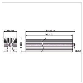
RF Solution offer a wide selection of Coaxial Fixed Termination (Dummy Load) for global customers. CT-500W-FA8056-NK-4G is Coaxial а Termination (Dummy Load) in Frequency Range of DC~4.0 GHz. It is made of high quality materials under a high standard, the Connector Type of this product is N-F (K), VSWR Max is 1.30 and Impedance is 50  $\Omega$ . The component has a good working performance and stability, it is ideal for handling a Power of 500 W.
