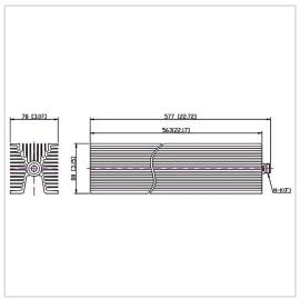
RF Solution offer a wide selection of Coaxial Fixed Termination (Dummy Load) for global customers. CT-500W-FA8056-NK-3G is a Coaxial Fixed Termination (Dummy Load) in Frequency Range of DC $\sim$ 3.0 GHz. It is made of high quality materials under a high standard, the Connector Type of this product is N-F (K), VSWR Max is 1.30 and Impedance is 50  $\Omega$ . The component has a good working performance and stability, it is ideal for handling a Power of 500 W.
