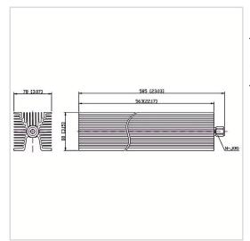
RF Solution offer a wide selection of Coaxial Fixed Termination (Dummy Load) for global customers. CT-500W-FA8056-NJ-6G is a Coaxial Fixed Termination (Dummy Load) in Frequency Range of DC~6.0 GHz. It is made of high quality materials under a high standard, the Connector Type of this product is N-M (J), VSWR Max is 1.45 and Impedance is 50  $\Omega$ . The component has a good working performance and stability, it is ideal for handling a Power of 500 W.
