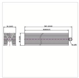
RF Solution offer a wide selection of Coaxial Fixed Termination (Dummy Load) for global customers. CT-500W-FA8056-NJ-4G is a Coaxial Fixed Termination (Dummy Load) in Frequency Range of DC~4.0 GHz. It is made of high quality materials under a high standard, the Connector Type of this product is N-M (J), VSWR Max is 1.30 and Impedance is 50  $\Omega$ . The component has a good working performance and stability, it is ideal for handling a Power of 500 W.
