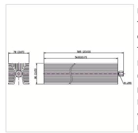
RF Solution offer a wide selection of Coaxial Fixed Termination (Dummy Load) for global customers. CT-500W-FA8056-NJ-3G is a Coaxial Fixed Termination (Dummy Load) in Frequency Range of DC~3.0 GHz. It is made of high quality materials under a high standard, the Connector Type of this product is DIN-F (K), VSWR Max is 1.30 and Impedance is 50  $\Omega$ . The component has a good working performance and stability, it is ideal for handling a Power of 500 W.
