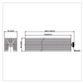
RF Solution offer a wide selection of Coaxial Fixed Termination (Dummy Load) for global customers. CT-500W-FA8056-DINK-6G is a Coaxial Fixed Termination (Dummy Load) in Frequency Range of DC $\sim$ 6.0 GHz. It is made of high quality materials under a high standard, the Connector Type of this product is DIN-F (K), VSWR Max is 1.45 and Impedance is 50  $\Omega$ . The component has a good working performance and stability, it is ideal for handling a Power of 500 W.
