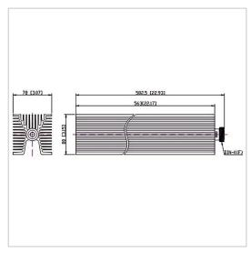
RF Solution offer a wide selection of Coaxial Fixed Termination (Dummy Load) for global customers. CT-500W-FA8056-DINK-4G is a Coaxial Fixed Termination (Dummy Load) in Frequency Range of DC~4.0 GHz. It is made of high quality materials under a high standard, the Connector Type of this product is DIN-F (K), VSWR Max is 1.30 and Impedance is 50  $\Omega$ . The component has a good working performance and stability, it is ideal for handling a Power of 500 W.
