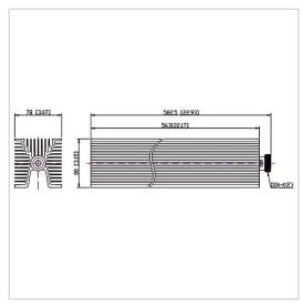
RF Solution offer a wide selection of Coaxial Fixed Termination (Dummy Load) for global customers. CT-500W-FA8056-DINK-3G is a Coaxial Fixed Termination (Dummy Load) in Frequency Range of DC $\sim$ 3.0 GHz. It is made of high quality materials under a high standard, the Connector Type of this product is DIN-F (K), VSWR Max is 1.30 and Impedance is 50  $\Omega$ . The component has a good working performance and stability, it is ideal for handling a Power of 500 W.
