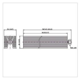
RF Solution offer a wide selection of Coaxial Fixed Termination (Dummy Load) for global customers. CT-500W-FA8056-DINJ-6G is a Coaxial Fixed Termination (Dummy Load) in Frequency Range of DC~6.0 GHz. It is made of high quality materials under a high standard, the Connector Type of this product is DIN-M (J), VSWR Max is 1.30 and Impedance is 50  $\Omega$ . The component has a good working performance and stability, it is ideal for handling a Power of 500 W.
