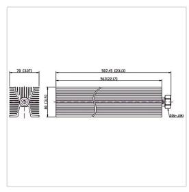
RF Solution offer a wide selection of Coaxial Fixed Termination (Dummy Load) for global customers. CT-500W-FA8056-DINJ-4G is a Coaxial Fixed Termination (Dummy Load) in Frequency Range of DC~4.0 GHz. It is made of high quality materials under a high standard, the Connector Type of this product is DIN-M (J), VSWR Max is 1.30 and Impedance is 50  $\Omega$ . The component has a good working performance and stability, it is ideal for handling a Power of 500 W.
