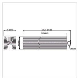
RF Solution offer a wide selection of Coaxial Fixed Termination (Dummy Load) for global customers. CT-500W-FA8056-DINJ-3G is a Coaxial Fixed Termination (Dummy Load) in Frequency Range of DC~3.0 GHz. It is made of high quality materials under a high standard, the Connector Type of this product is DIN-M (J), VSWR Max is 1.30 and Impedance is 50  $\Omega$ . The component has a good working performance and stability, it is ideal for handling a Power of 500 W.
