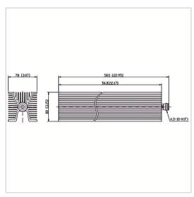
RF Solution offer a wide selection of Coaxial Fixed Termination (Dummy Load) for global customers. CT-500W-FA8056-4310K-6G is a Coaxial Termination (Dummy Load) in Frequency Range of DC~6.0 GHz. It is made of high quality materials under a high standard, the Connector Type of this product is 4.3-10-F (K), VSWR Max is 1.45 and Impedance is 50  $\Omega$ . The component has a good working performance and stability, it is ideal for handling a Power of 500 W.
