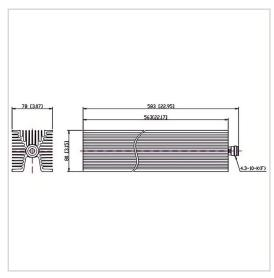
RF Solution offer a wide selection of Coaxial Fixed Termination (Dummy Load) for global customers. CT-500W-FA8056-4310K-4G is a Coaxial Fixed Termination (Dummy Load) in Frequency Range of DC~4.0 GHz. It is made of high quality materials under a high standard, the Connector Type of this product is 4.3-10-F (K), VSWR Max is 1.30 and Impedance is 50  $\Omega$ . The component has a good working performance and stability, it is ideal for handling a Power of 500 W.
