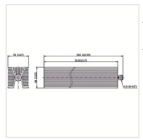
RF Solution offer a wide selection of Coaxial Fixed Termination (Dummy Load) for global customers. CT-500W-FA8056-4310K-3G is a Coaxial Fixed Termination (Dummy Load) in Frequency Range of DC~3.0 GHz. It is made of high quality materials under a high standard, the Connector Type of this product is 4.3-10-F (K), VSWR Max is 1.30 and Impedance is 50  $\Omega$ . The component has a good working performance and stability, it is ideal for handling a Power of 500 W.
