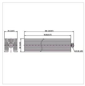
RF Solution offer a wide selection of Coaxial Fixed Termination (Dummy Load) for global customers. CT-500W-FA8056-4310J-6G is a Coaxial Termination (Dummy Load) in Frequency Range of DC~6.0 GHz. It is made of high quality materials under a high standard, the Connector Type of this product is 4.3-10-M (J), VSWR Max is 1.45 and Impedance is 50  $\Omega$ . The component has a good working performance and stability, it is ideal for handling a Power of 500 W.
