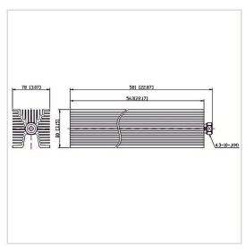
RF Solution offer a wide selection of Coaxial Fixed Termination (Dummy Load) for global customers. CT-500W-FA8056-4310J-4G is a Coaxial Fixed Termination (Dummy Load) in Frequency Range of DC~4.0 GHz. It is made of high quality materials under a high standard, the Connector Type of this product is 4.3-10-M (J), VSWR Max is 1.30 and Impedance is 50  $\Omega$ . The component has a good working performance and stability, it is ideal for handling a Power of 500 W.
