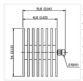
RF Solution offer a wide selection of Coaxial Fixed Termination (Dummy Load) for global customers. CT-30W-RA5442-2.92K-40G is a Coaxial Fixed Termination (Dummy Load) in Frequency Range of DC~40.0 GHz. It is made of high quality materials under a high standard, the Connector Type of this product is 2.92-F (K), VSWR Max is 1.30 and Impedance is 50  $\Omega$ . The component has a good working performance and stability, it is ideal for handling a Power of 30 W.
