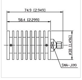
RF Solution offer a wide selection of Coaxial Fixed Termination (Dummy Load) for global customers. CT-30W-RA3858-SJ-26.5G is a Coaxial Fixed Termination (Dummy Load) in Frequency Range of DC~26.5 GHz. It is made of high quality materials under a high standard, the Connector Type of this product is SMA-M (J), VSWR Max is 1.50 and Impedance is 50  $\Omega$ . The component has a good working performance and stability, it is ideal for handling a Power of 30 W.
