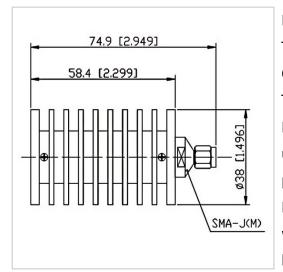
RF Solution offer a wide selection of Coaxial Fixed Termination (Dummy Load) for global customers. CT-30W-RA3858-SJ-18G is a Coaxial Fixed Termination (Dummy Load) in Frequency Range of DC~18.0 GHz. It is made of high quality materials under a high standard, the Connector Type of this product is SMA-M (J), VSWR Max is 1.35 and Impedance is 50  $\Omega$ . The component has a good working performance and stability, it is ideal for handling a Power of 30 W.
