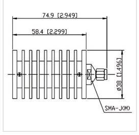
RF Solution offer a wide selection of Coaxial Fixed Termination (Dummy Load) for global customers. CT-30W-RA3858-SJ-12.4G is а Coaxial Termination (Dummy Load) in Frequency Range of DC~12.4 GHz. It is made of high quality materials under a high standard, the Connector Type of this product is SMA-M (J), VSWR Max is 1.30 and Impedance is 50  $\Omega$ . The component has a good working performance and stability, it is ideal for handling a Power of 30 W.
