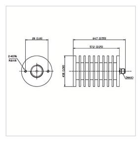
RF Solution offer a wide selection of Coaxial Fixed Termination (Dummy Load) for global customers. CT-30W-RA3857-SK-8G is a Coaxial Fixed Termination (Dummy Load) in Frequency Range of DC~8.0 GHz. It is made of high quality materials under a high standard, the Connector Type of this product is SMA-F (K), VSWR Max is 1.30 and Impedance is 50  $\Omega$ . The component has a good working performance and stability, it is ideal for handling a Power of 30 W.
